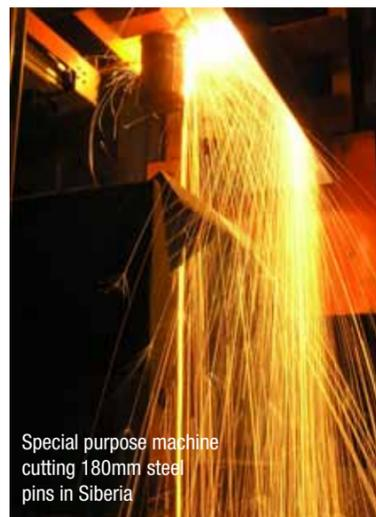
Special purpose machine cutting 180mm steel pins in Siberia
